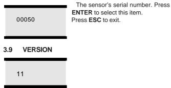
Version numbers of the transmitter's electronics and software. Press **ENTER** to select this item. Press **ESC** to exit. With the **UP/DOWN**[ $\uparrow\downarrow$ ] keys you can select either **CPU HW, CPU SW, ADC HW, ADC SW** or **MAN REV** (manual revision) revision number or **CPU ID**-number from this submenu.
