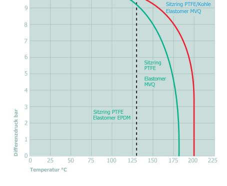
These limits apply to the intended use. Process variables and characteristics of the medium can influence the values of the diagram. Temperatures below 0 °C upon request.
