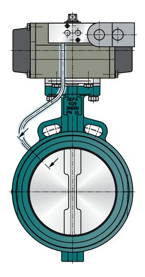
The butterfly valves with inflatable seat ring are preferably used for the shut-off, discharge and dosing of abrasive bulk materials.
