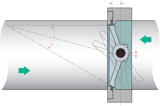
The triple offset butterfly and regulating valves are the advancement of the double offset technology.
