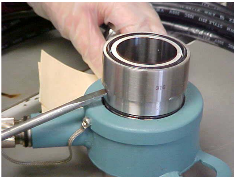
Figure 24. Removal of First Toroid Sleeve from the Toroid Assembly
