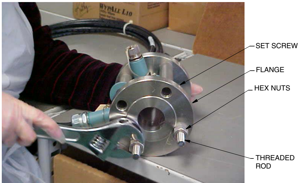
Figure 22. Removing the Hex Nuts
