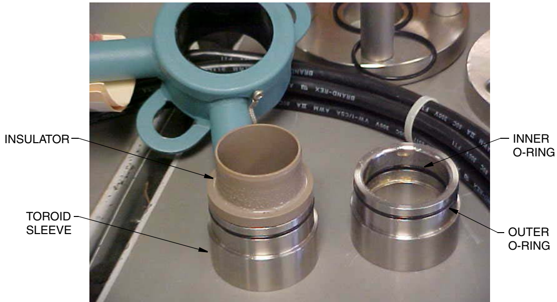
Figure 25. Removal of Second Toroid Sleeve and Insulator from Toroid Assembly
