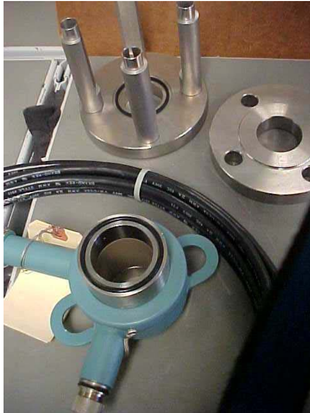
Figure 23. Separation of Flanges from the Toroid Assembly
