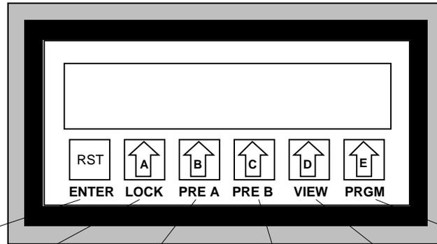
Press to RESET in operating mode; Press to "ENTER" in programming mode.
