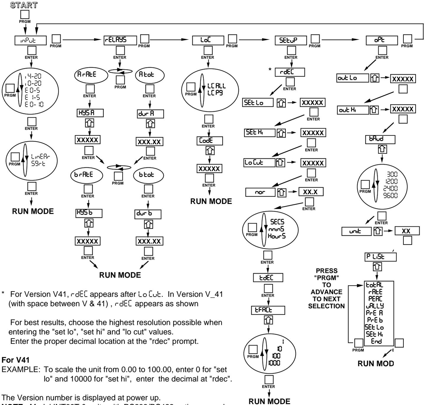
\* For Version V41, rdEC appears after LoCut. In Version V\_41 (with space between V & 41), rdEC appears as shown
