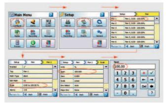
Example of a recorder menu path from the Main Menu to Pen Scale configuration with clear and rapid navigation
